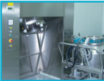
UNLOADING SIDE - BIO-SEAL FRAME + UNLOADING INTO SEALED CONTAINERS
