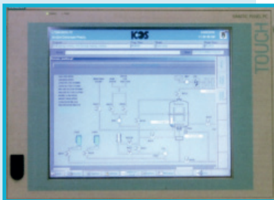
OP or PC: SIEMENS or ALLEN-BRADLEY SCADA SYSTEM DESIGNED FOR FDA 21 CFR PART 11
