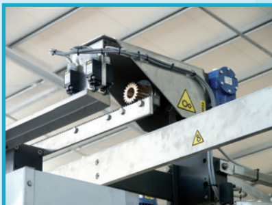
DETAIL OF DOORS MOVEMENT
